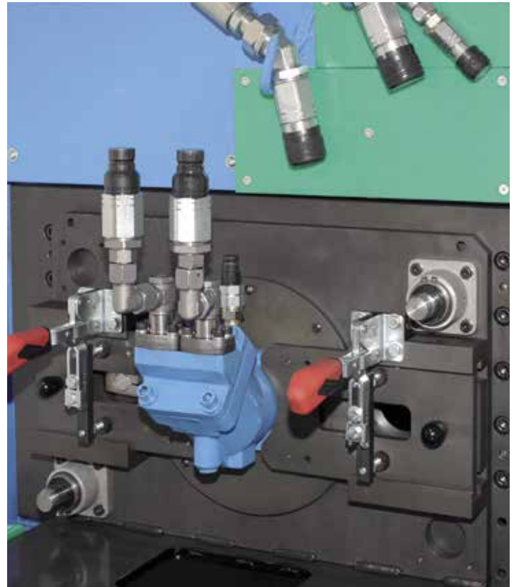
test bench for motors
